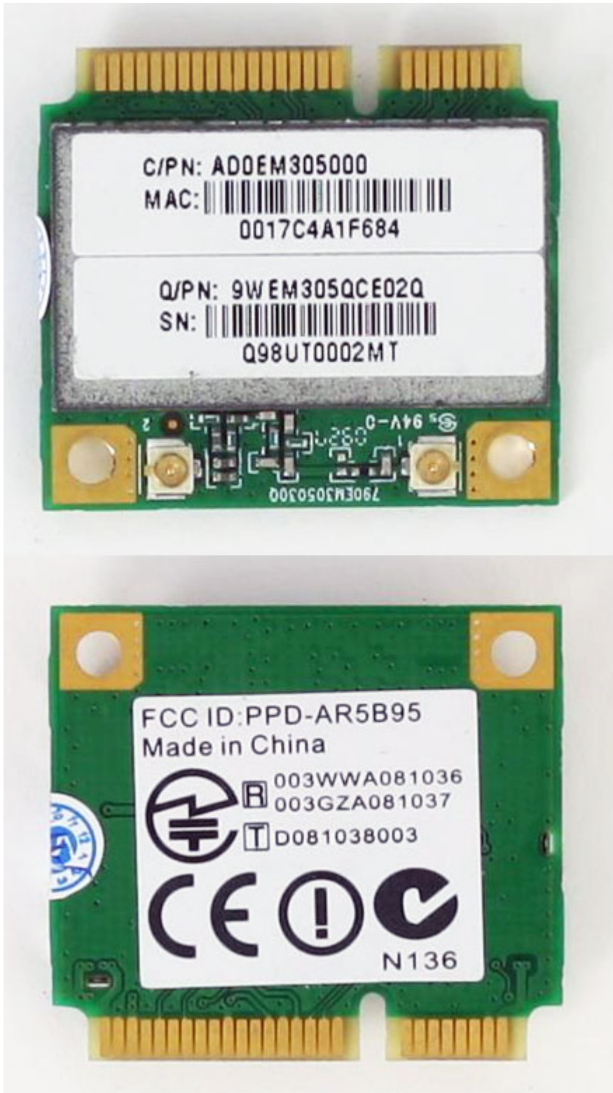
Wireless LAN Mini-PCI Express card Azurewave AW-NE785H Atheros AR9280 / AR5B95 chipset (802.11b/g/n)
